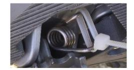
2: Assemble the kit. Install the rear footpeg, return spring, M8 footpeg pivot bolt, and M8 washer in both brackets. Important, see picture: The flat washer should be installed below the rear footpeg. The air gap between the bracket ant the top of the footpeg is intended. These design features are there to ensure smooth operation of the footpeg fold back safety feature.
