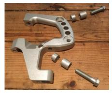
the upper holes (see picture) If swapped, the upper bolt end will collide with the swingarm.
